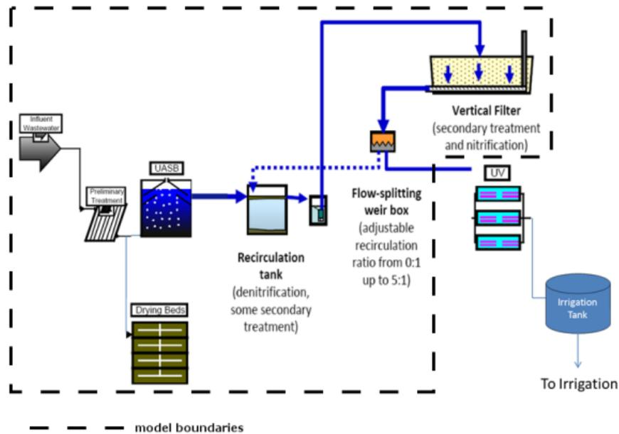
Figure 2: Vertical flow constructed wetland with model boundaries for CEA [BDZ, 2012]
