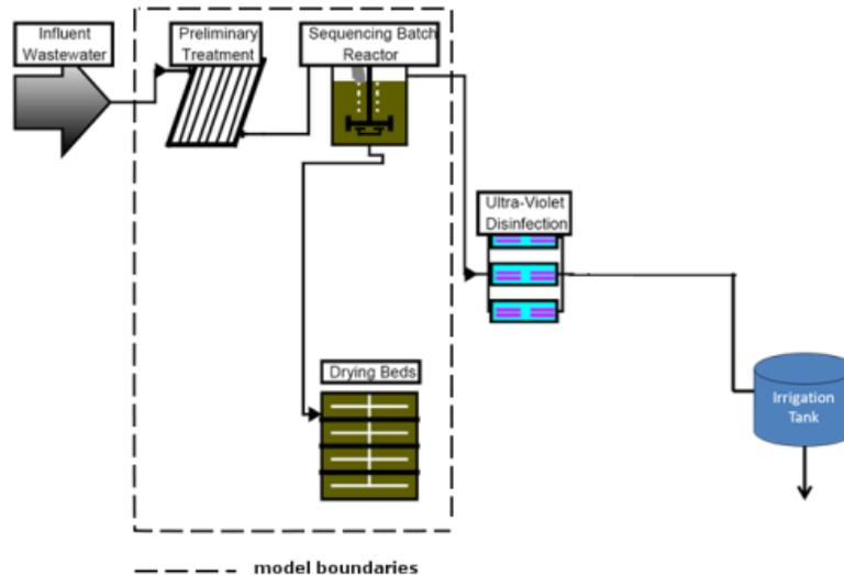
Figure 1: Sequencing batch reactor with model boundaries for CEA [BDZ, 2012]
